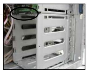
4. From the front side, secure the right side of the cage with two screws.
